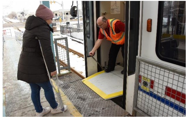
Figure 18: A Blue Line TRAX operator lowering the ramp for the passenger in crutches
