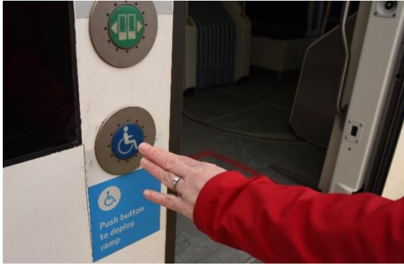
Figure 17: A person pushing the blue wheelchair button on the TRAX door to deploy the ramp.
